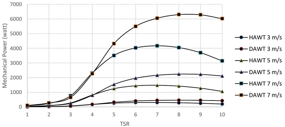
Figure 3. Mechanical Power of Wind Turbines Rotor
