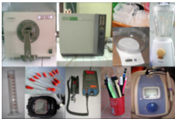
Figure 1. (a) Spectrophotometer; (b) Incubator; (c) Plastic containers; (d) Scale; (e) Blender; (f) Measuring cup; (g) Pipettes; (h) Stopwatch; (i) Micromotor; (j) Stationery; (k) Ultrasonic scaler
