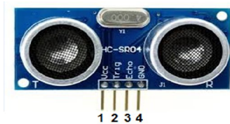
Vcc- Connects to 5V of positive voltage for power Trig- A pulse is sent here for the sensor to go into ranging mode for object detection Echo- The echo sends a signal back if an object has been detected or not. If a signal is returned, an object has been detected. If not, no object has been detected. GND- Completes electrical pathway of the power.
