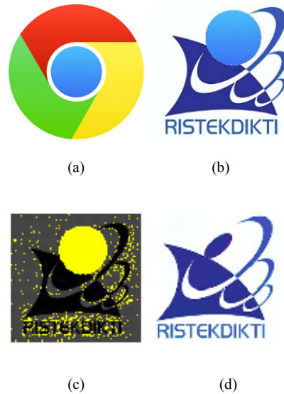
Fig. 6. Test collage attack of proposed method (a) chrome logo ; (b) tampered image (c) tamper detection; (d) recovered image
