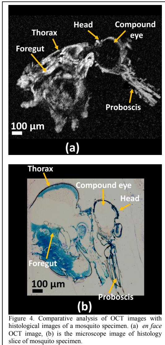
Figure 4. Comparative analysis of OCT images with histological images of a mosquito specimen. (a) en face OCT image, (b) is the microscope image of histology slice of mosquito specimen.
