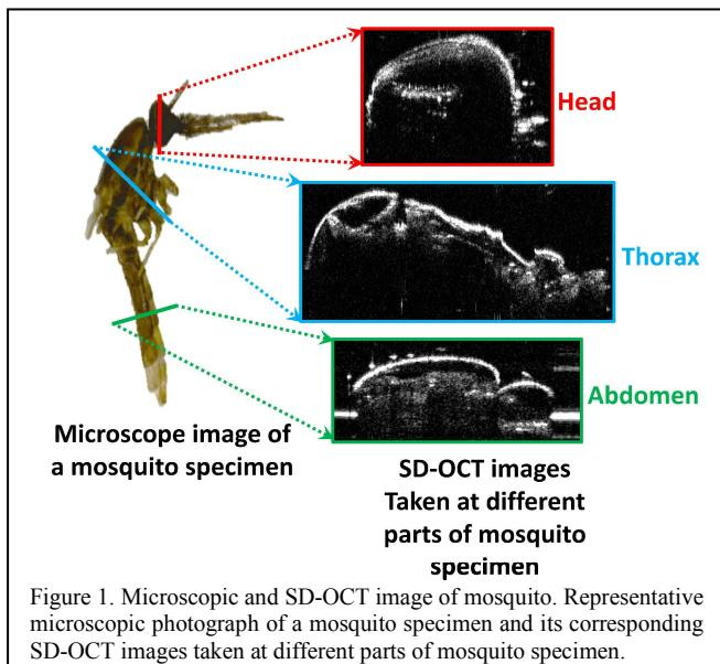
A representative image of a mosquito specimen is shown in figure 1. After being anesthetized, specimens were carefully separated and stored. The experimental environment was maintained at 23 °C and 50% humidity. OCT imaging was carried out immediately after the specimens were anesthetized. For experimental convenience, the wings and the legs were clipped carefully without damaging other parts of the specimen.
