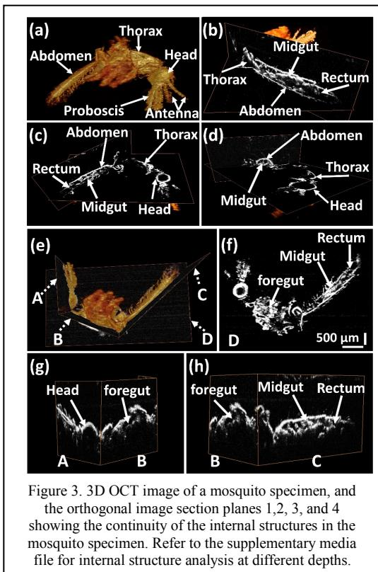
Figure 3. 3D OCT image of a mosquito specimen, and the orthogonal image section planes 1,2, 3, and 4 showing the continuity of the internal structures in the mosquito specimen. Refer to the supplementary media file for internal structure analysis at different depths.
