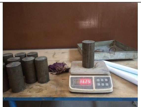
Penimbangan Sampel Beton
