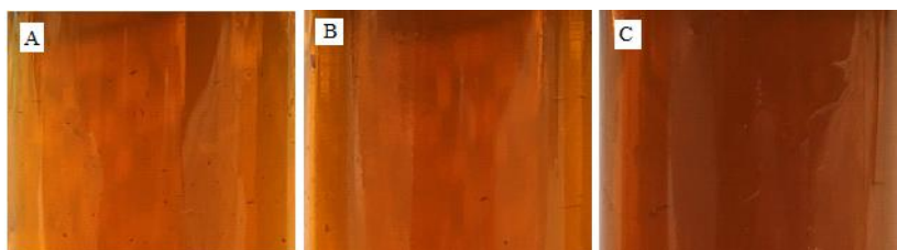
174 175 Fig. 5. Apparent color of mixture with 50:50 compositions of patchouli oil 176 (Aceh Besar) with (a) kerosene (b) palm oil and (c) lubricant oil SAE 40. 177 From the figure we can see there is no significant different among them 178
