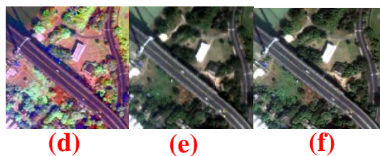
Fig.3. Original and pan-sharpened images: (a) Original MS image, and (c)-(f) results of different pan-sharpening methods, (b) HIS, (c) CN-Spectral (d) CN-Brovey, (E) PCA, and (F) GS.
