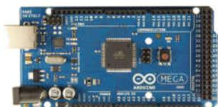
Gambar 1. Arduino Mega 2560
