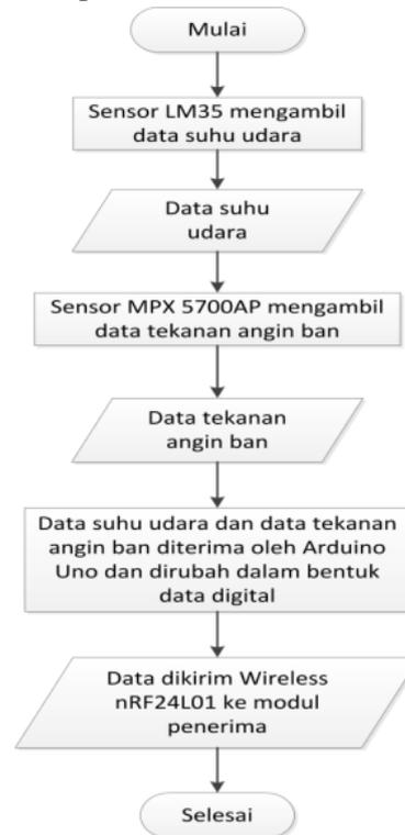
Gambar 13. *Flowchart* Modul Sensor
