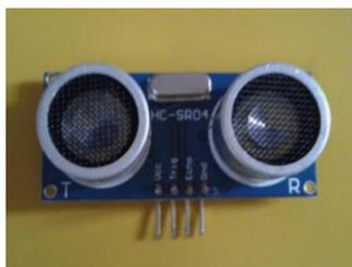
Gambar 4. Sensor Ultrasonik HC-SR04
