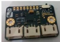
Gambar 1. Sensor Accelerometer MMA7361
