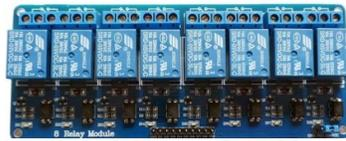
Gambar8. 8 Channel RelayModule
