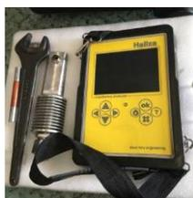
**Gambar 2. Diesel Engine Analyzer HALIZA 8.4**
