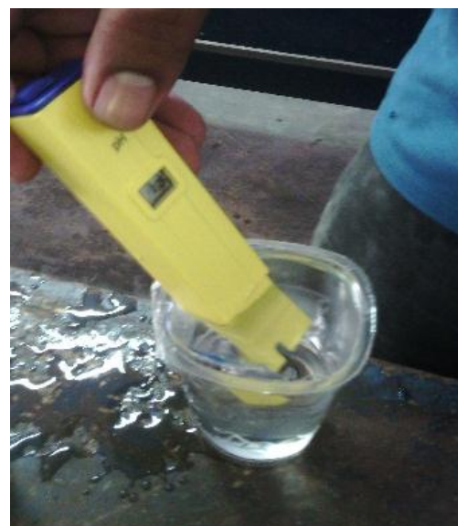
Gambar 2. Pengujian Kadar pH Air Mineral
