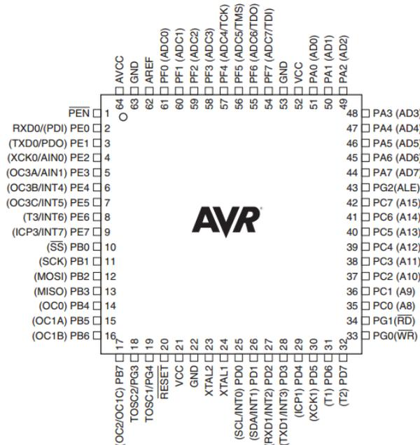
Gambar 2. Konfigurasi Pin Atmega128 [3]
