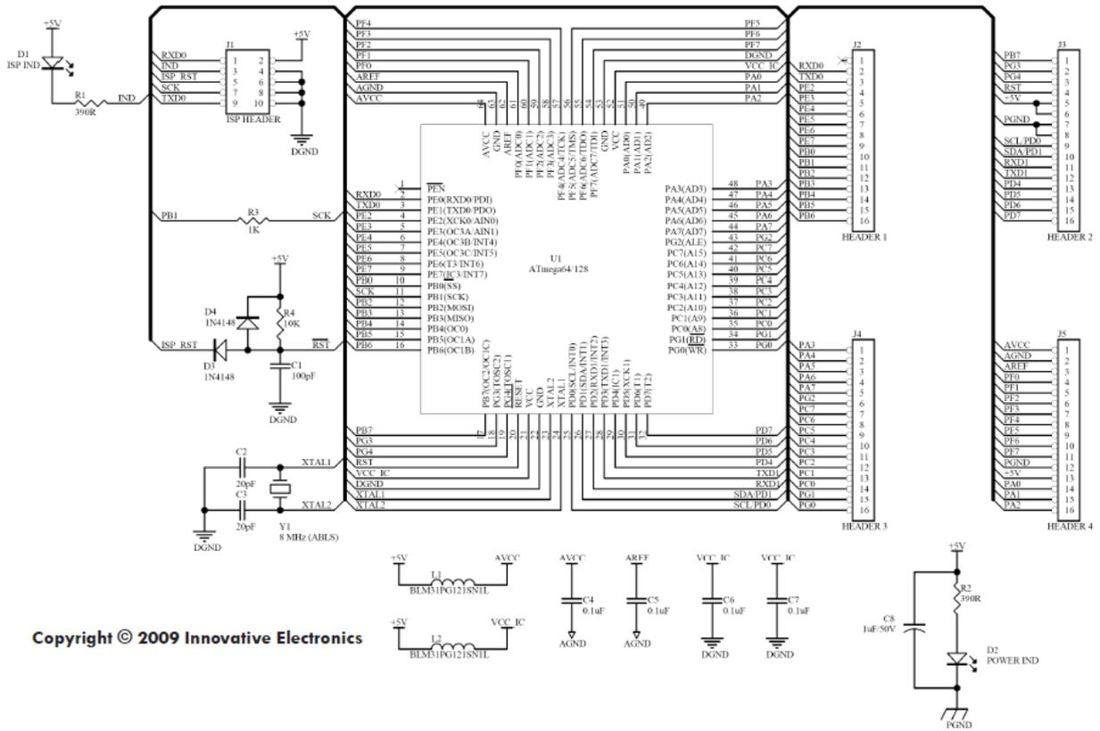
Gambar 7. Rangkaian DT-AVR ATMEGA 128 CPU Module [6]
