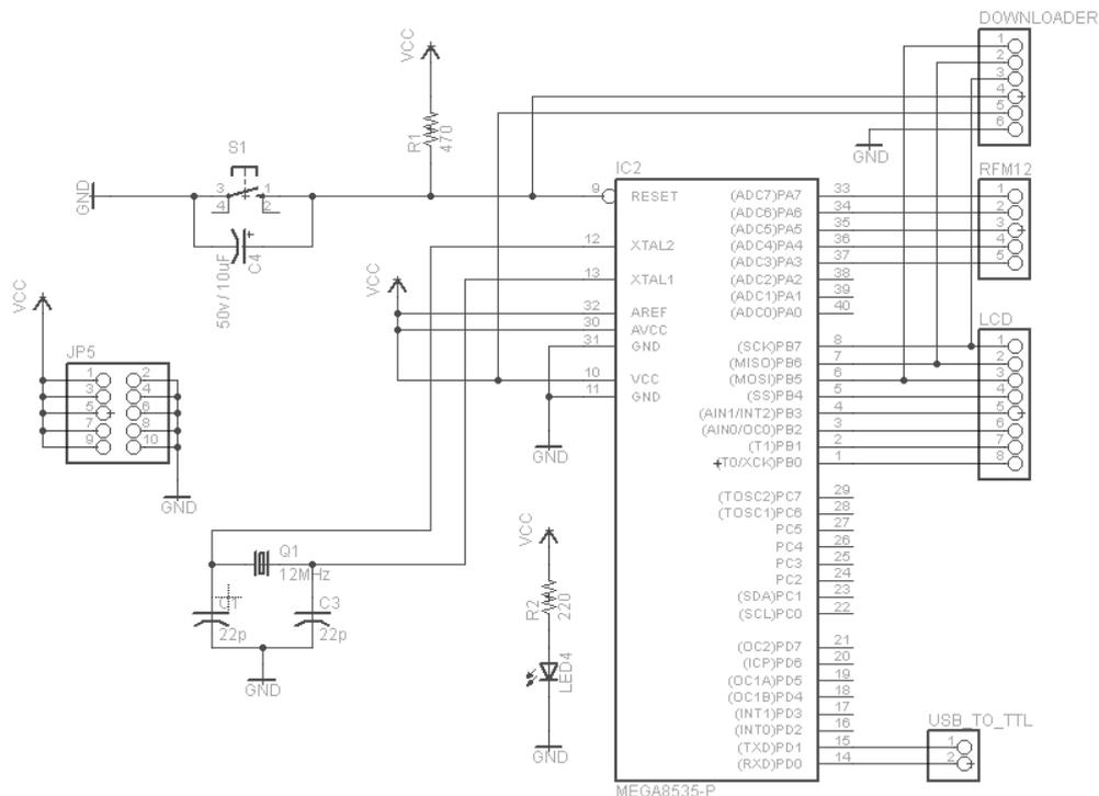
Gambar 11. Rangkaian Minimum Sistem Atmega 8535 Central Unit
