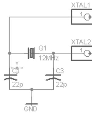
Gambar 9. Rangkaian Osilator Atmega 8535 Central Unit.
