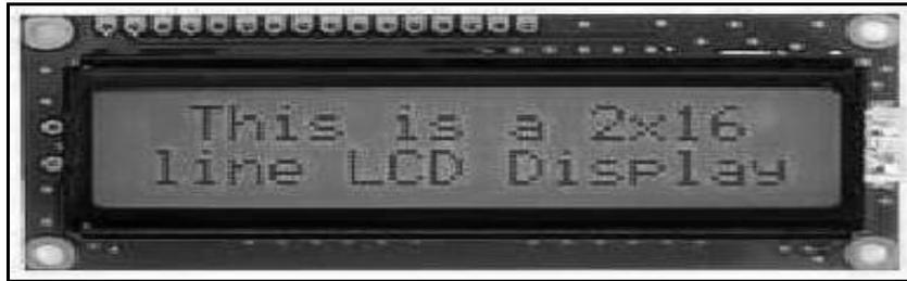
Gambar 4. LCD 16x2 [5]
