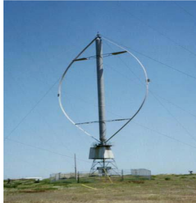
Gambar 4: Turbin angin tipe Darrieus Sumber : Wikipedia, http://wikipedia.org
