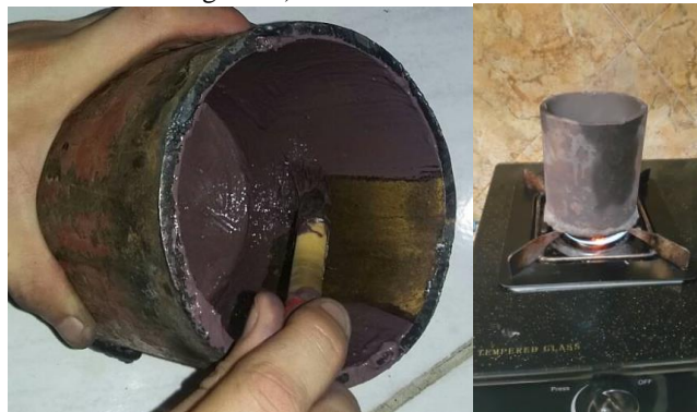
Figure 1. Coating application process on crucible (left) and heating process of crucible (right)
